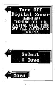
You can turn the digital sonar off, however this also turns all automatic features off also, such as auto sensitivity, auto ranging, and Fish I.D.
